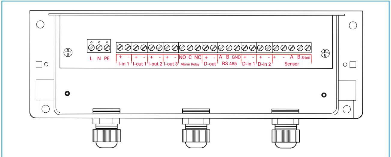
Fig. 11: Electrical connection of the MSE 300-FH
