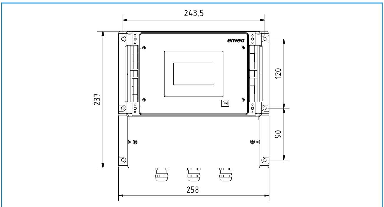
Fig. 7: Dimension of the MSE 300-FH (front view)
