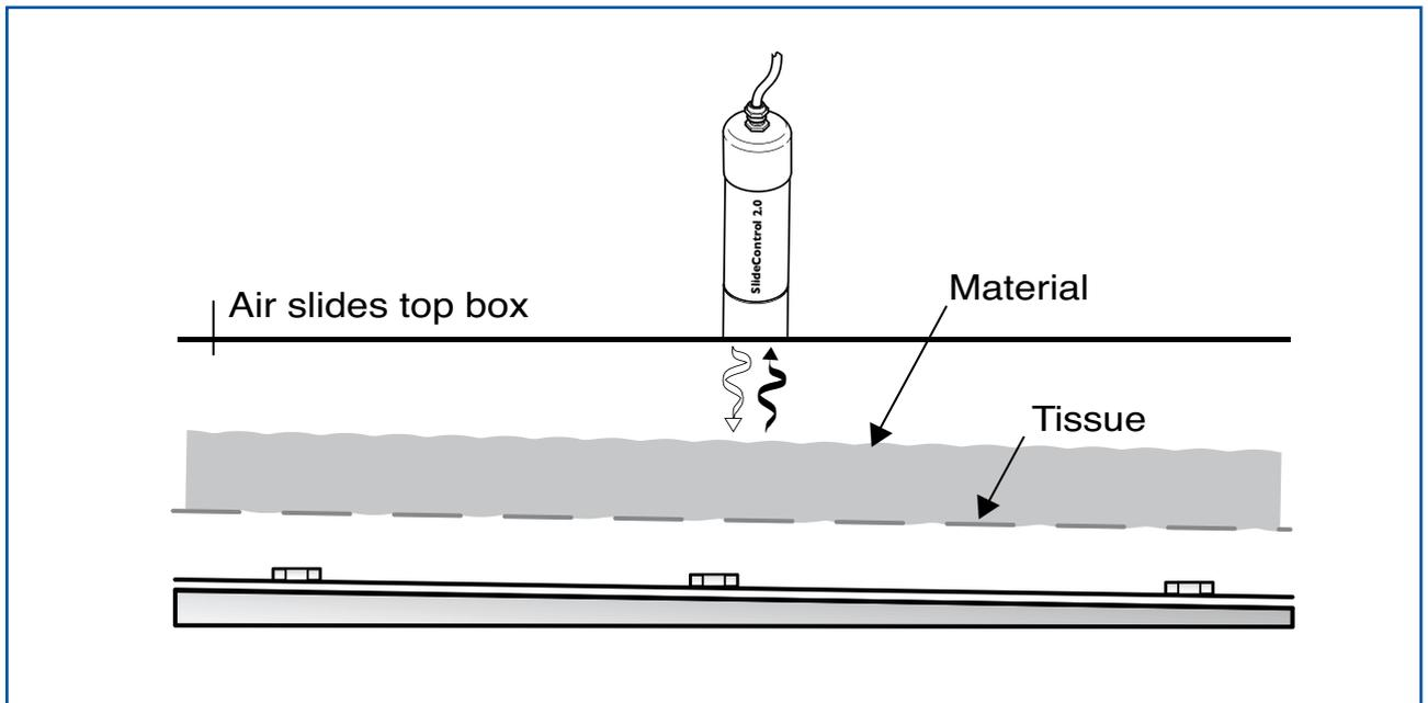
Fig. 3: Coupling and reflection of the microwave
