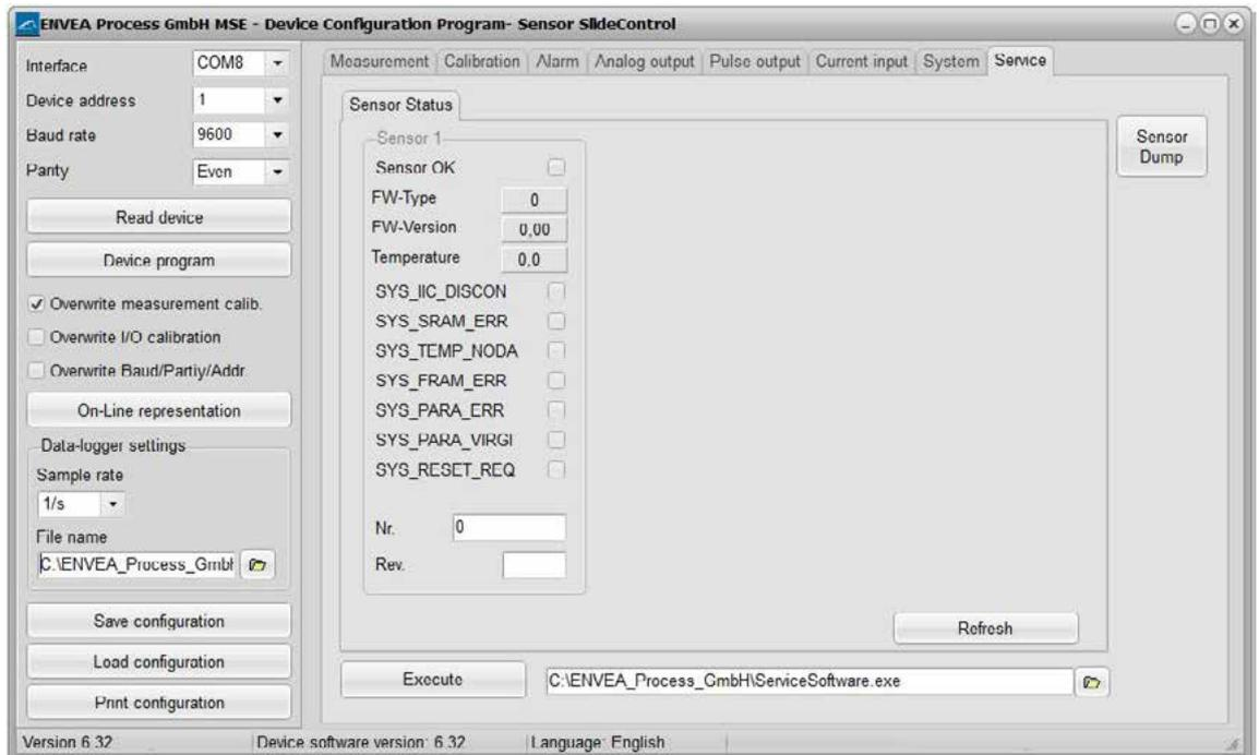
The status of each connected sensor is displayed in menu **9. Service**. FW type, FW version, temperature, serial number and possible hardware errors are automatically read and displayed.
