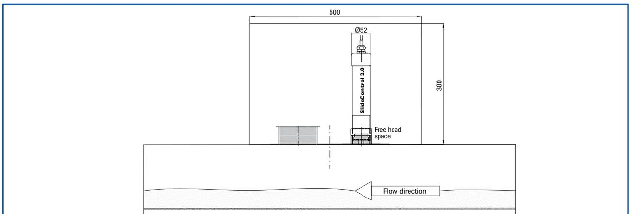
Fig. 5: Built in situation SlideControl 2.0
