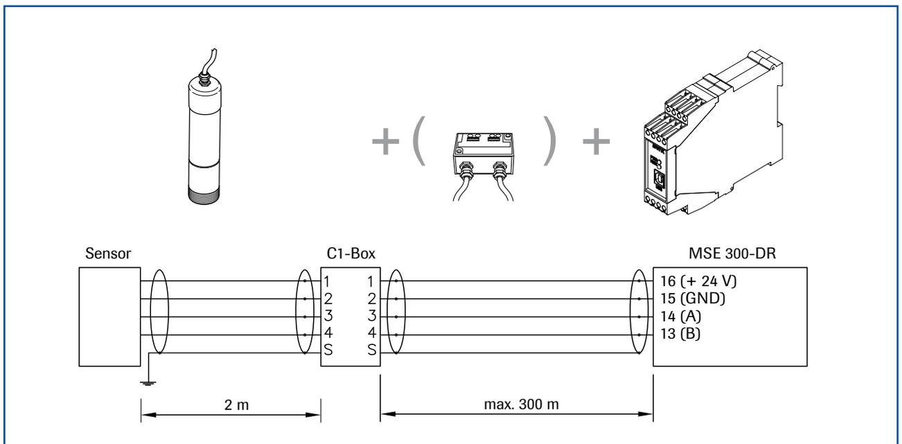
Fig. 1: Overview with C1-Box and MSE 300 in the DIN Rail housing
