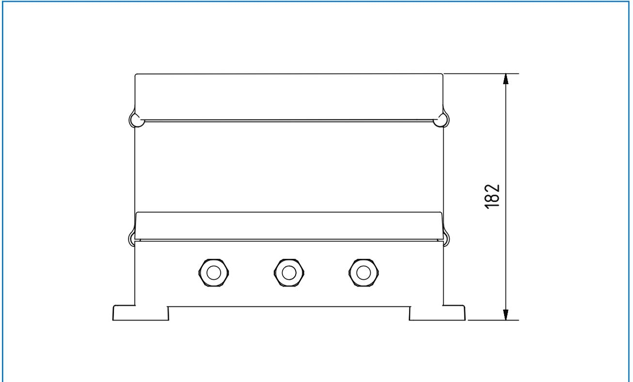
Fig. 8: Dimension of the MSE 300-FH (side view)
