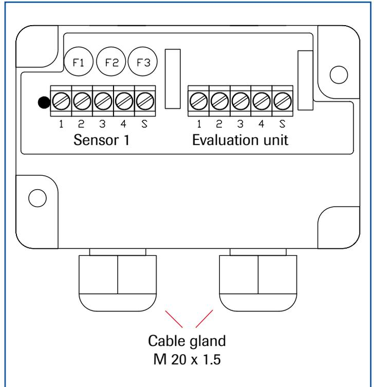
Fig. 12: Electrical connection for the C1-Box
