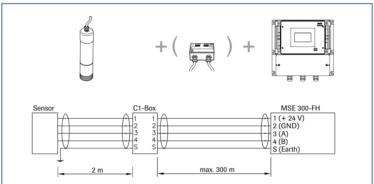
Fig. 2: Overview with C1-Box and MSE 300 in the field housing
