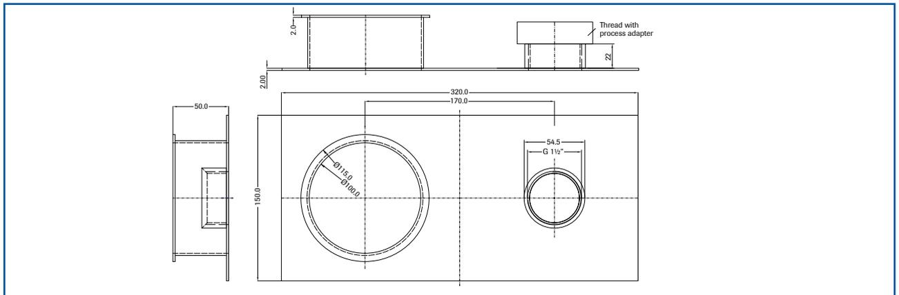
Fig. 4: Dimension of mounting plate
