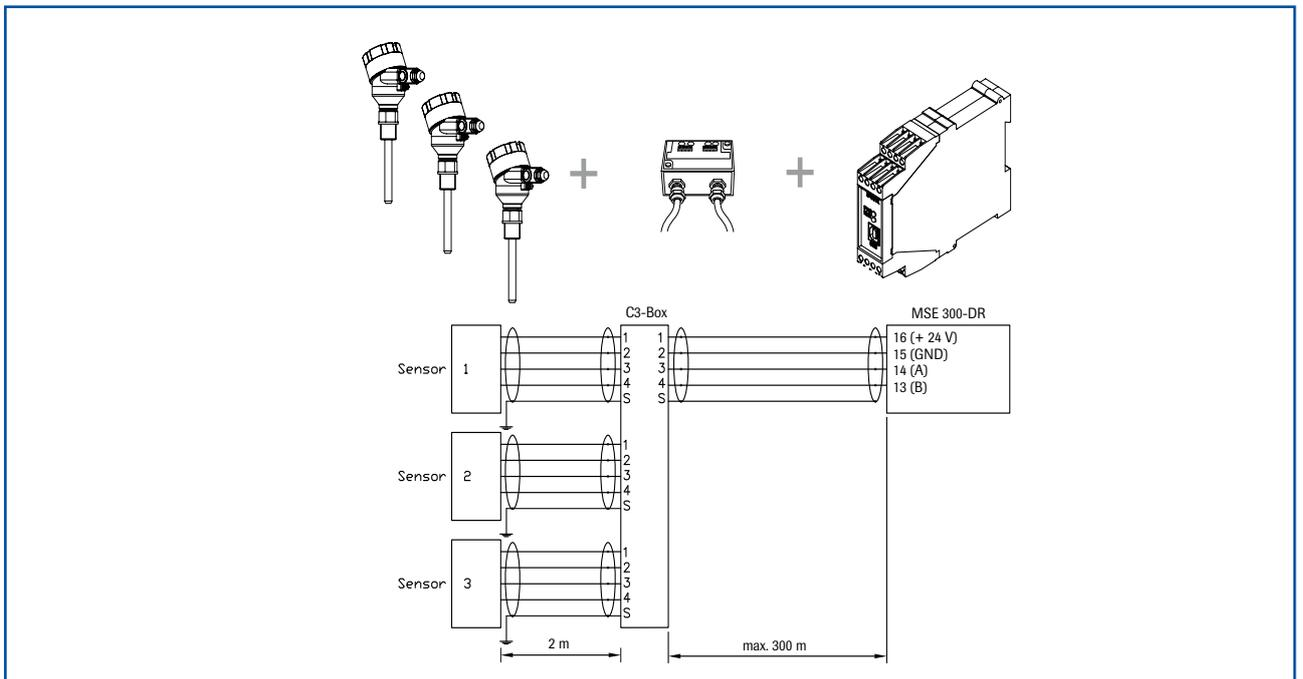
Fig. 4: Overview with C3-Box and MSE 300 in the DIN Rail housing
