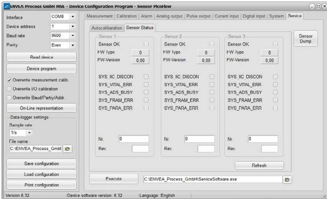
The status of each connected sensor is displayed in menu **9. Service**. FW type, FW version, temperature, serial number and possible hardware errors are automatically read and displayed. In the case of a display exchange, the contrast could be changed via the PC software.
