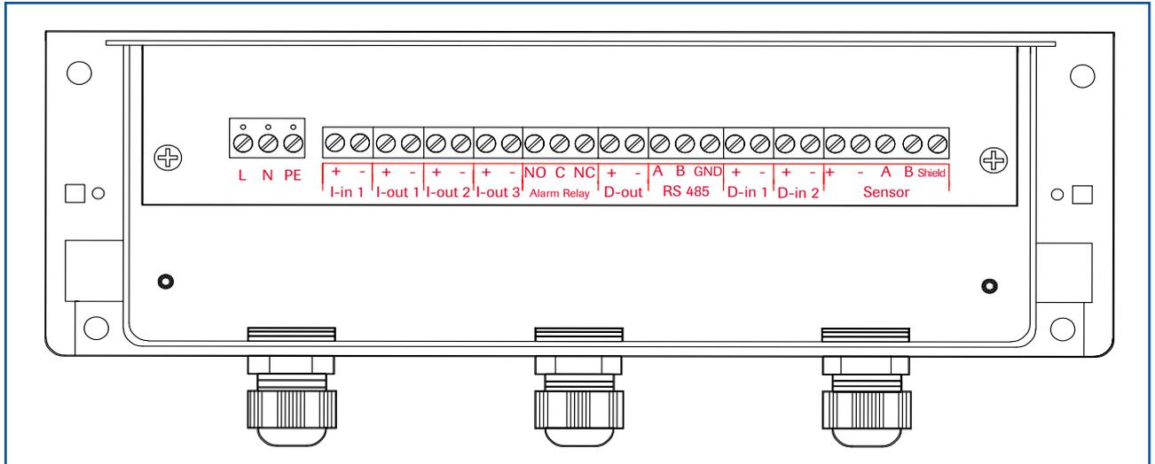
Fig. 15: Electrical connection of the MSE 300-FH
