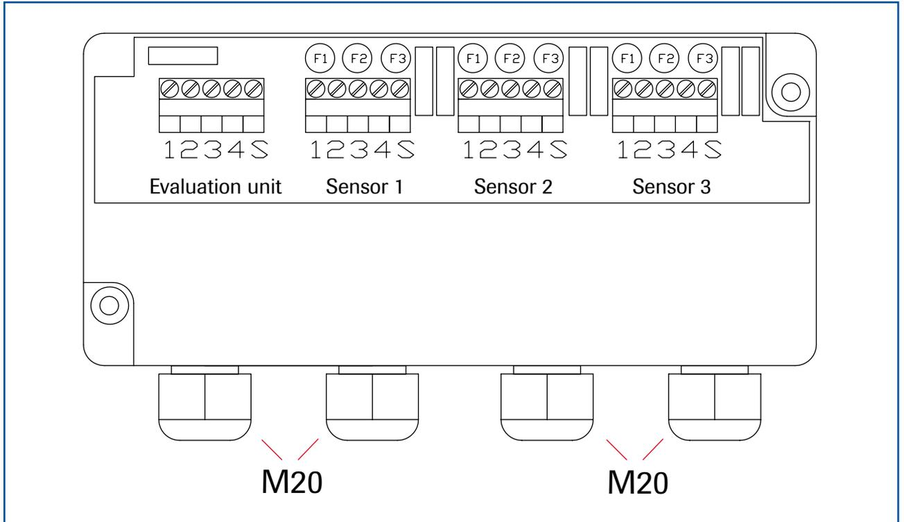
Fig. 16: Electrical connection for the C3-Box
