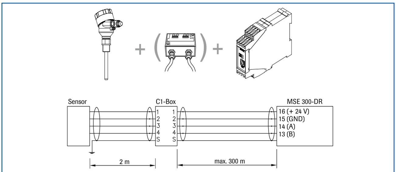
Fig. 2: Overview with C1-Box and MSE 300 in the DIN Rail housing
