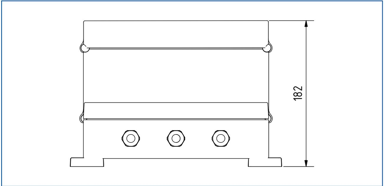
Fig. 9: Dimension of the MSE 300-FH (side view)
