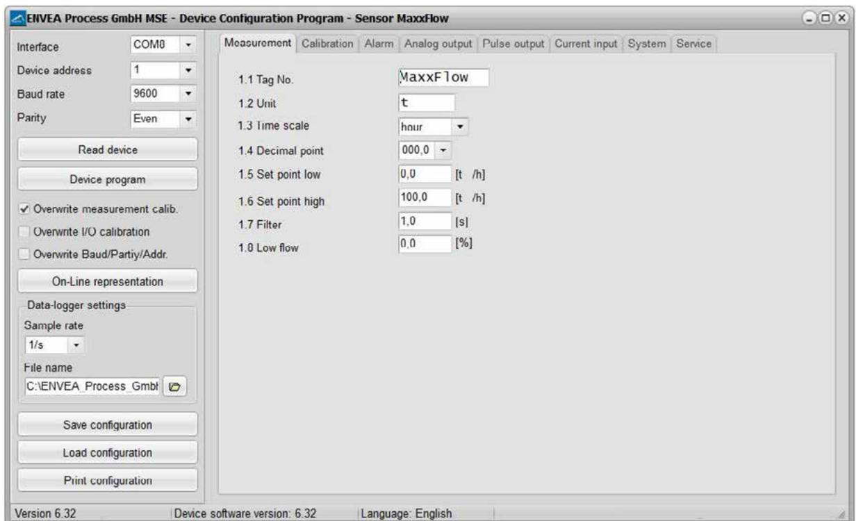
Communication is established by clicking on “Read device”. The acknowledgement message “Parameter read in” is displayed. If an error message is displayed instead, check the communication parameters and cable connections between the PC and the transmitter.
