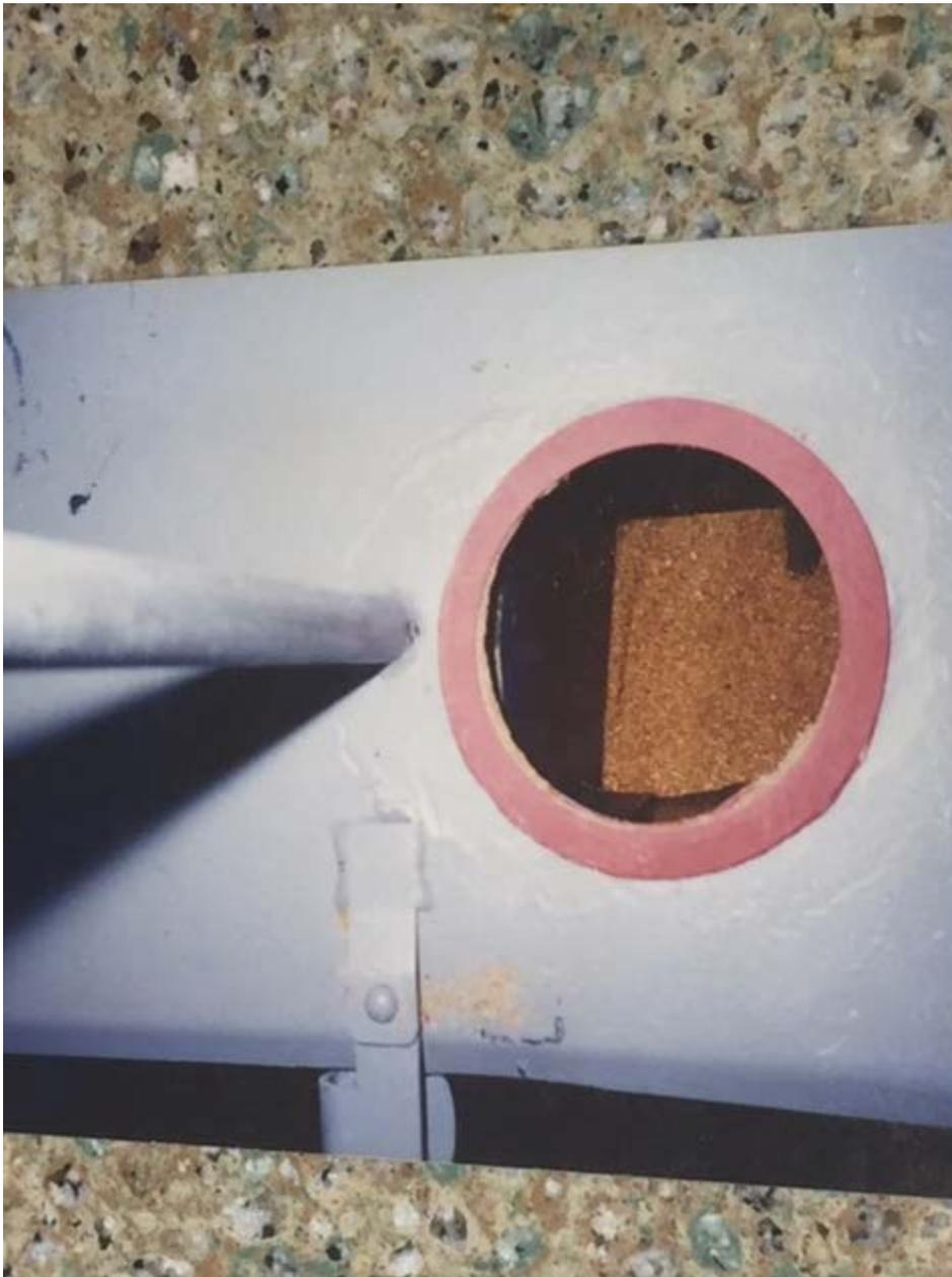
If the auger is visible to the ENVEA system, this may negatively impact the results of the measurement. If this is the case, it is recommended to cut out a section of the auger where the ENVEA is measuring product (see Figure 17 - Screw conveyor measurement location).
