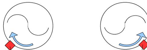
Do not install the sensor under or on the side of the screw, it must be installed mid-size from bottom, on the side where material is pushed up (depending rotation side of the screw). (Approximattly 30° from the screw bottom).
