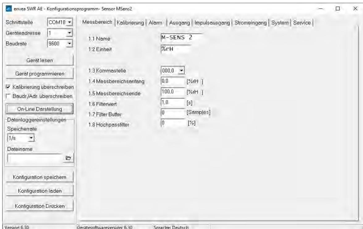
Communication is established by clicking on “Read device”. The acknowledgement message “Parameter read in” is displayed. If an error message is displayed instead, check the communication parameters and cable connections between the PC and the Evaluation unit.
