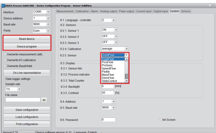
In the menu „System“, under „Sensor“ (8.2.5 or 7.2.5), the correct sensor must be selected.
