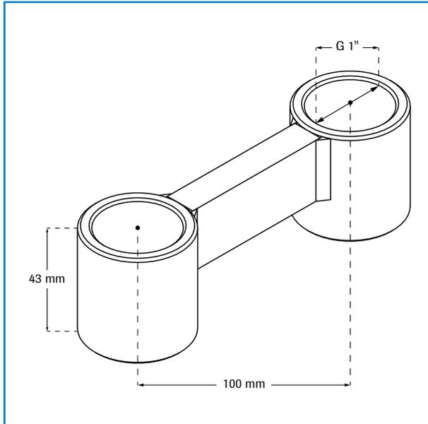
Fig. 12: Dimensions G 1" double socket
