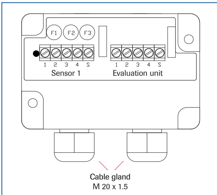
Fig. 19: Electrical connection C1-Box
