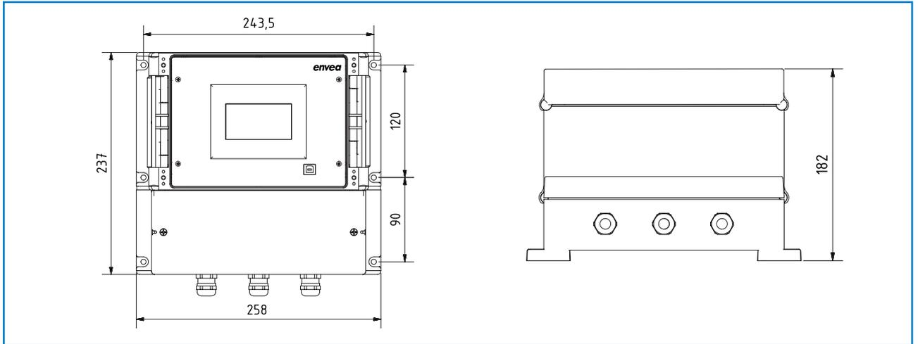
Fig. 9: Dimensions of the MSE 300-FH
