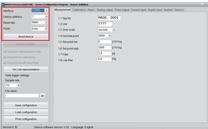
Select the correct COM port and connect to the device using the „read device“ button.
