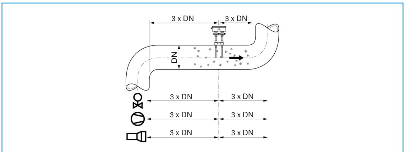
Fig. 6: Recommended distances to valves, etc. (DN = nominal diameter)
