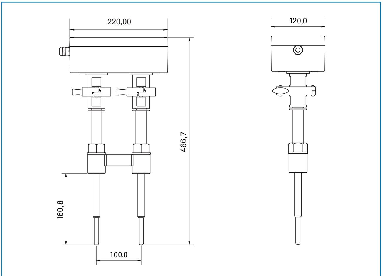
Fig. 14: Dimensions AirFlow P sensor
