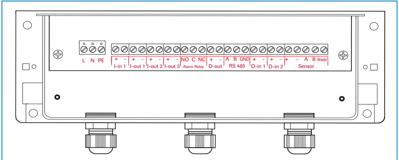
Fig. 17: Electrical connection of the MSE 300-FH
