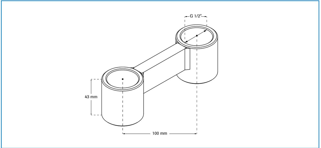
Fig. 15: Dimension G 1/2" double socket
