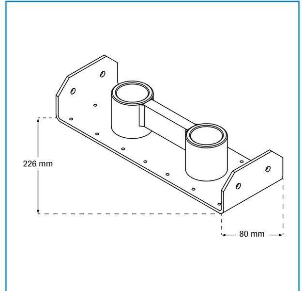
Abb. 13: Dimensions G 1"-double-screw on-socket for thin channels
