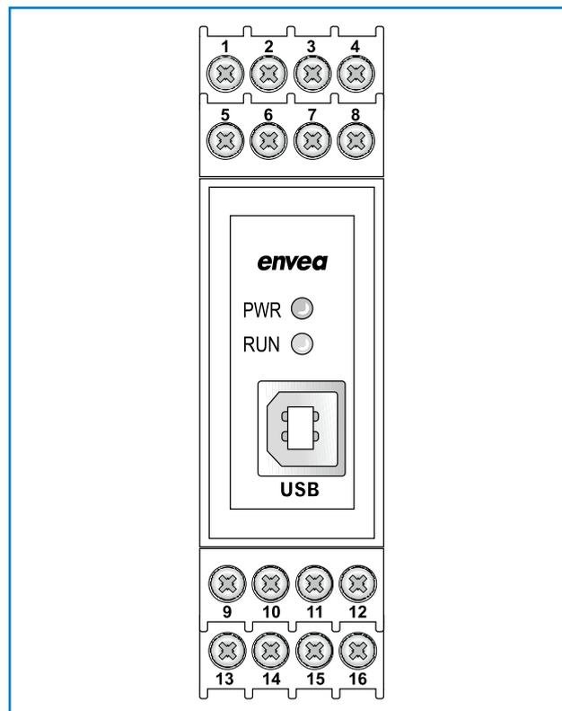
Fig. 15: Electrical connection of the MSE 300-DR
