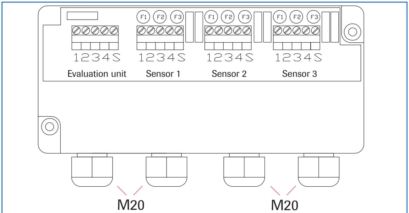
Fig. 18: Electrical connection C3-Box
