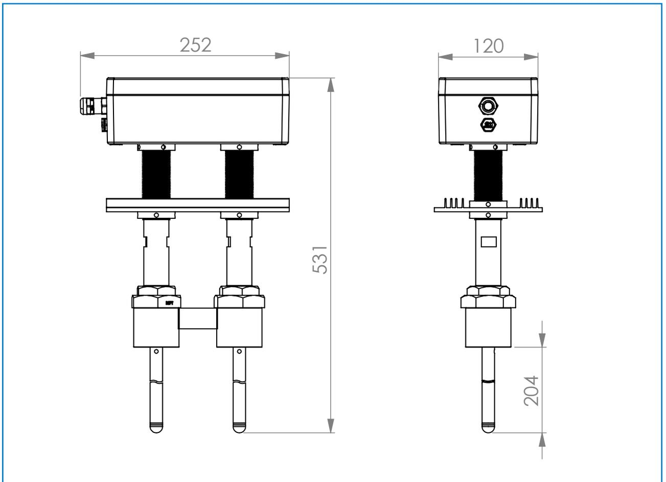
Fig. 16: Dimension AirFlow P-HT sensor
