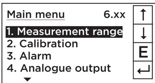
To enter the main menu, the display must be switched to button at any point for several seconds. The selection of submenus appears.
