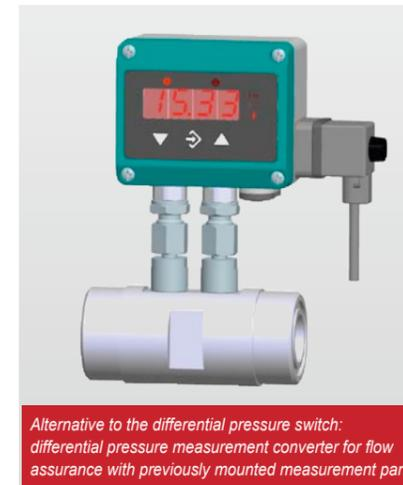
of the medium. If the minimum circulation volume of the heat carrier is not achieved, the switch contact blocks the hot waste gas to ensure the flow. This ensures that the pipes in the boiler are protected and overheating is avoided.
