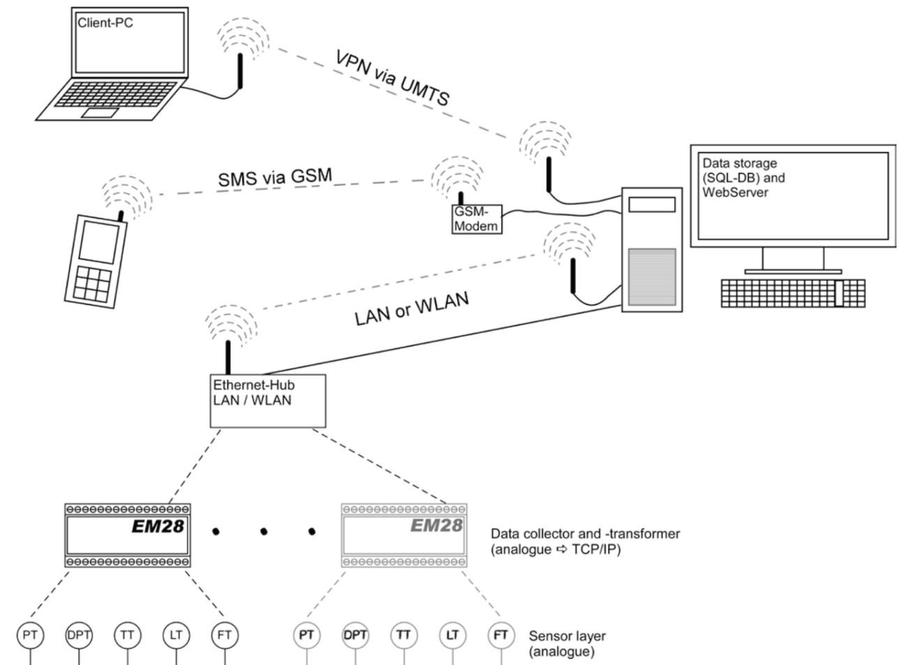
Wireless transmission of measurement signals is available for particularly difficult to reach measurement points.
