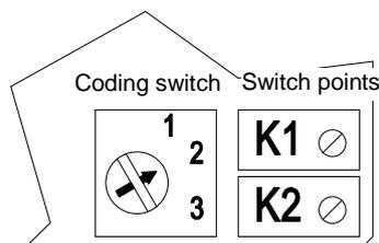
The coding switch can be used to set the value that is to be displayed.
